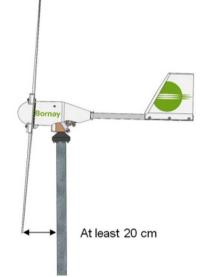
Once the wind turbine has been installed on the tower, check that it can turn freely and that there are no obstacles within the diameter of the blades.
