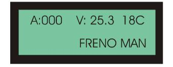
When the manual braking switch is activated, this is indicated on the screen at the end of the second line and the brake indication LED is also illuminated.
