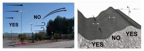
To maximize the performance of your wind turbine, it should be installed as far as possible from the obstruction and atop a tower higher point from this obstacle.
